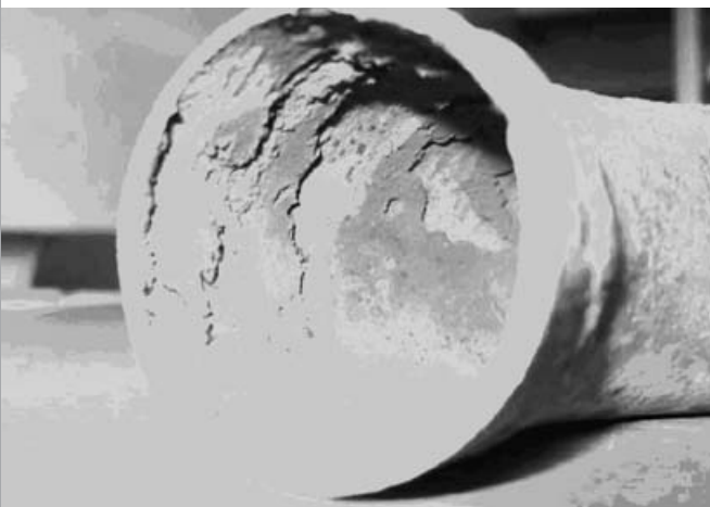
Figure 2: Pipe corrosion caused by carbonic acid
