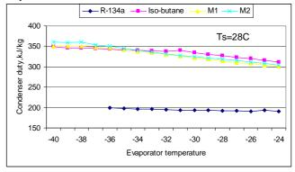
Figure 11 effect of evaporator temperature on condenser duty
