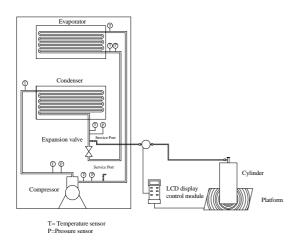
Figure 3 Schematic diagram of the charging system
