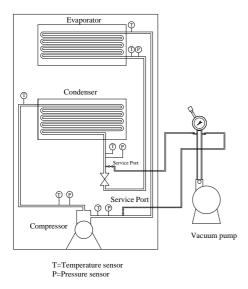
Figure 2 Schematic diagram of the evacuation system
