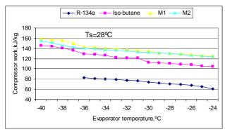
Figure 9 effect of evaporator temperature on work of compression for R-134a
