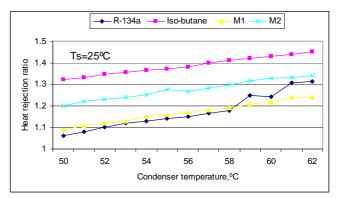
Figure 12 Heat rejection ratio at different condensing temperature
