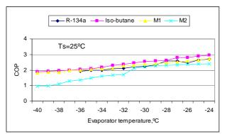
Figure 4 Effect of inlet refrigerant on co-efficient of performance
