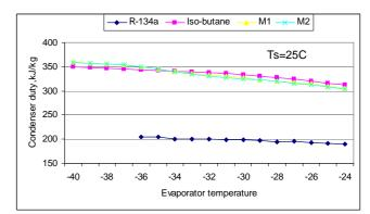
Figure 10 effect of evaporator temperature on condenser duty
