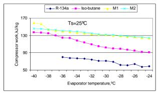
Figure 8 effect of evaporator temperature on work of compression for R-134a
