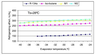
Figure 7 refrigerating effect versus inlet evaporator temperature
