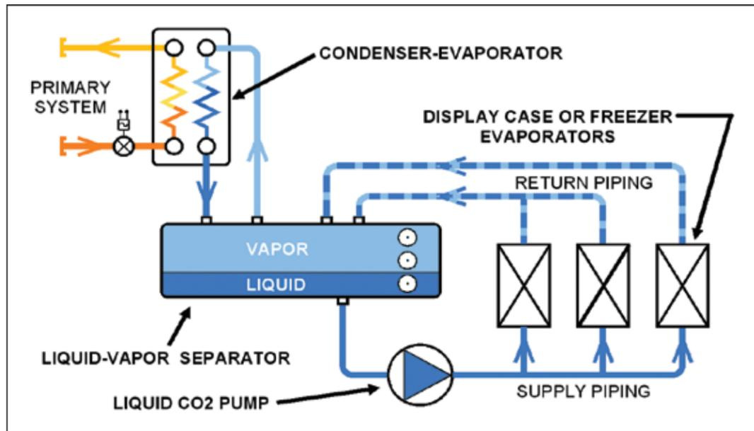
Heat is absorbed in the display case through evaporator coils similar to those used in traditional DX systems. The CO<sub>2</sub> does not completely evaporate in the coil and is returned to a separator as a mixture of liquid and vapor. The liquid portion of the CO<sub>2</sub> in the separator is available to be pumped to the display
